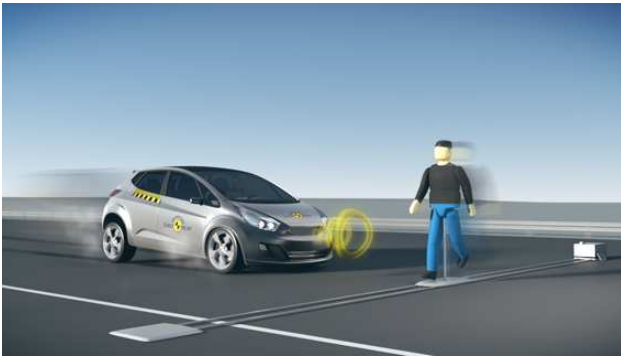
Figure 12. AEB: Cameras are the major sensor
