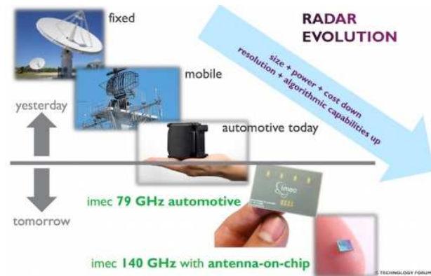
Figure 27. Efforts are underway to develop higher-bandwidth automotive radar systems
