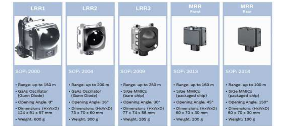
Figure 26. Bosch's radar sensor evolution, in terms of weight and measurement distance/angle
