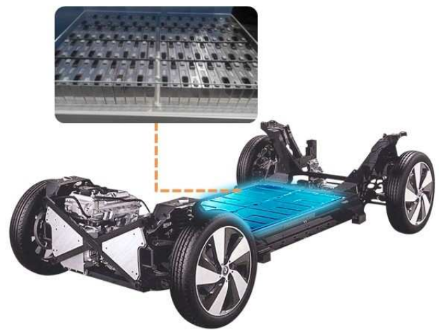
Figure 245. Samsung SDI's battery packs installed in BMW i3
