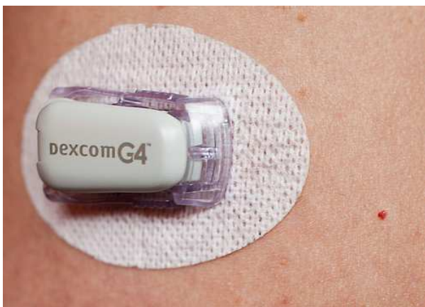
Figure 24. Application of transmitter and sensor
