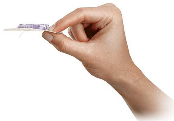
Figure 23. 13-14mm subcutaneous sensor measures glucose levels
