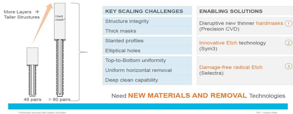
Figure 4. Significant challenges expected for 96-layer or over 3D NAND
